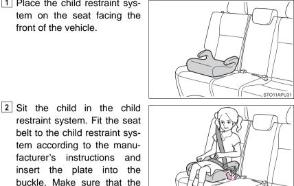
Check that the shoulder belt is correctly positioned over the child's shoulder and that the lap belt is as low as possible. ( $\rightarrow$ P. 26)
