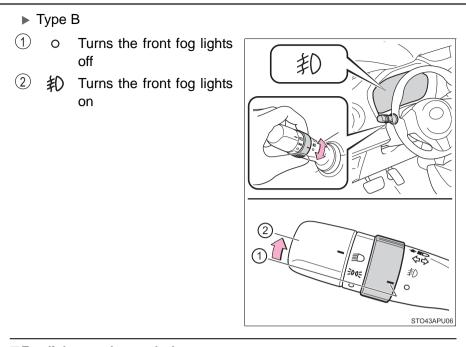
**Fog lights can be used when** The headlights are on in low beam.
