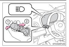
You can flash the high beams with the headlights on or off.
