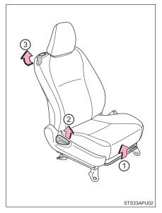
Moving front passenger's seat for rear seat entry (3-door models only)
