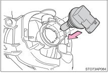
7 Turn and secure the bulb. Install the connector.
