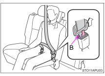
2 To release the hooked plate "A", insert the plate "B", the key into the hole on the buckle.
