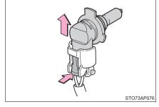
3 Replace the light bulb, and install the bulb base.
