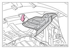
4 Unplug the connector while pressing the lock release.
