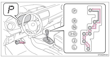
While the engine switch is in the "ON" position, move the shift lever with the brake pedal depressed.
