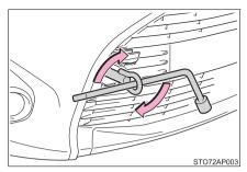
5 Securely attach a cable or chain to the towing eyelet.
