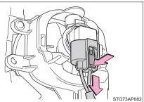
5 Turn the bulb base counterclockwise and remove.
