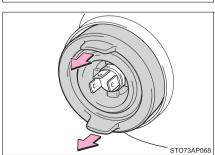
3 Release the bulb retaining spring.
