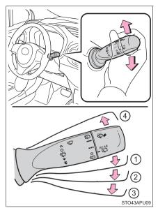
(5) Washer/wiper dual operation The wiper will automatically operate a couple of times after the washer squirts.
