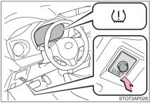
5 Wait for a few minutes with the engine switch in the "ON" position and then turn the engine switch to the "LOCK" position.
