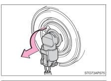
2 Pull the bulb out while pressing the lock release of the connector.
