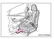
When a booster seat is installed, always ensure that the shoulder belt is positioned across the center of the child's shoulder. The belt should be kept away from the child's neck, but not so that it could fall off the child's shoulder. Failure to do so may result in death or serious injury in the event of a sudden braking, sudden swerving or an accident.
